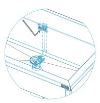
Screw on the,overflow with M6x25 cylinder head screw (allen screw)
