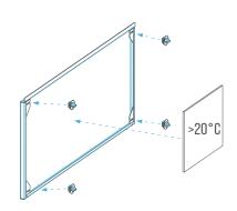
1. glue pads inside 2. install clips in panels
