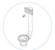
Discard the slotted screw with countersunk.
