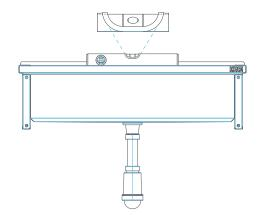
Check slope and correct if necessary. No accessibility after orifice assembly].
