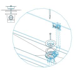
Screw the drain strainer to the drain valve
