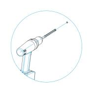
12mm drill diameter, min 7cm deep 2x blow out drill hole and clean with the wire brush
